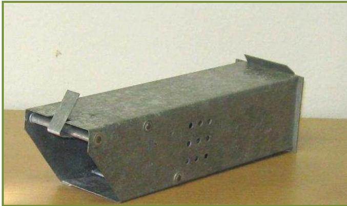
Figure 1 - Rödl live trap (245x60x60 mm).
