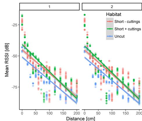
**Figure 3** – Relationship between RSSI and distance for two habitat types and 5 loggers (all with epoxy applied). Points indicate raw measurements in different habitats, ribbons indicate predicted relationship between RSSI and distance returned from the model, pale ribbon indicates the 95% simultaneous confidence intervals.
